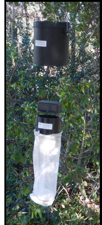
CO 2 traps lure many species of mosquitoes with dry ice, mimicking the smell of an exhaling animal. These traps are set overnight.
